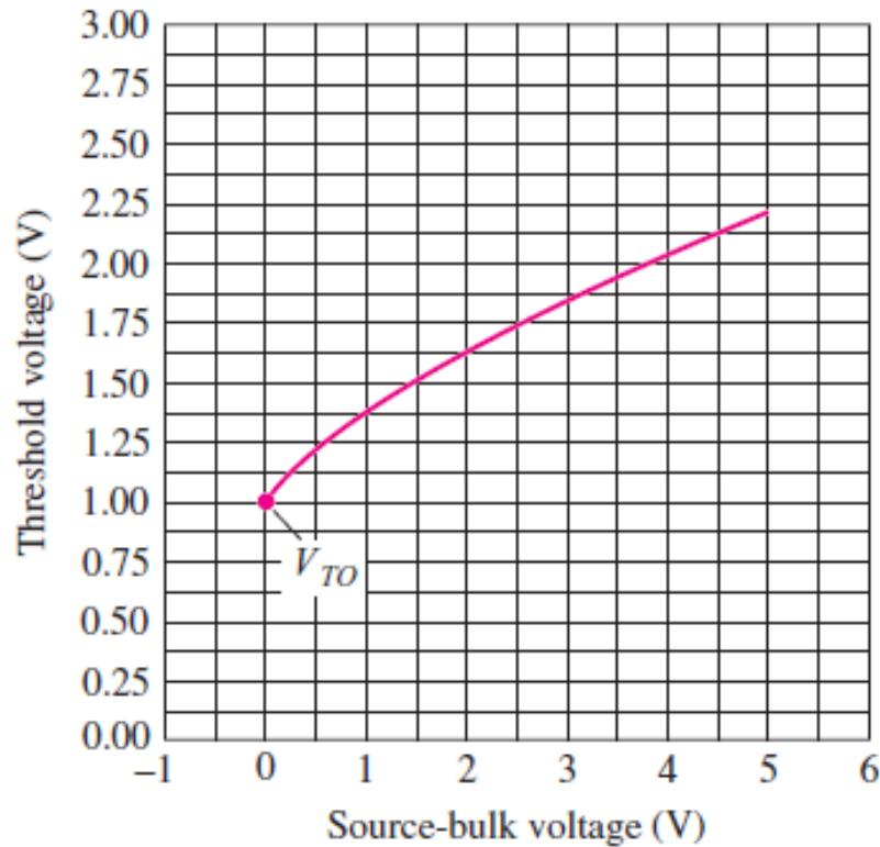
$$V_{TN} = V_{TO} + \gamma(\sqrt{v_{SB} + 2\phi_F} - \sqrt{2\phi_F})$$
